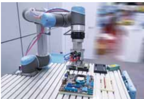
A pneumatic robot arm assembles electronic parts on a computer circuit board.
