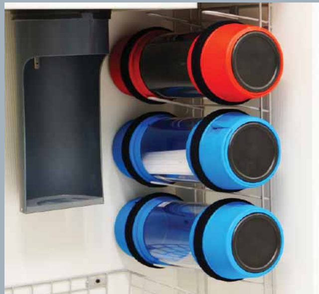
Modern pneumatic tubes operate on exactly the same principle as their historic counterparts. A motor either forces air into the tube to push a canister or sucks air out to create vacuum which pulls the canister to its destination.
