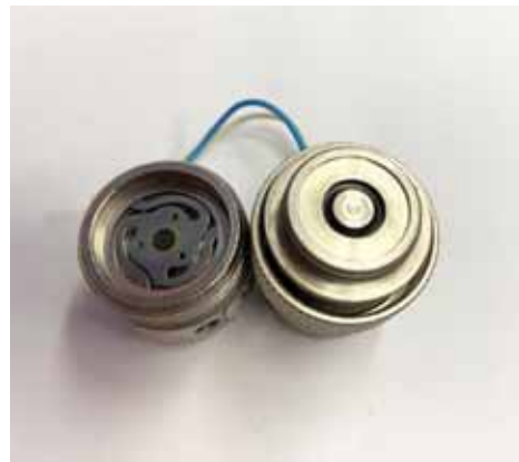
An internal view of a typical pneumatic solenoid valve. The curled piece on the left moves up and down to allow or stop flow. The spider is inverted to show rubber valve seat.
