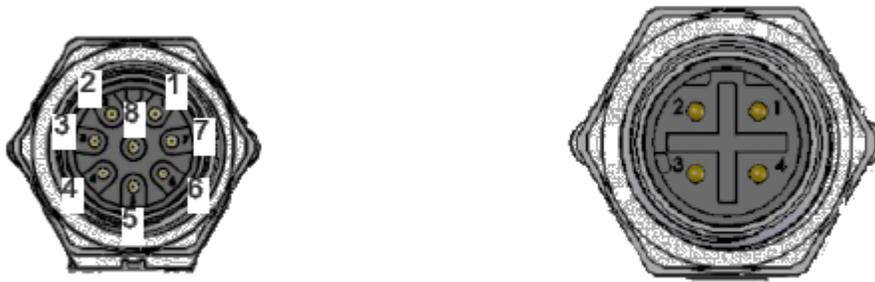
**Figure 1 Power and network connectors**
