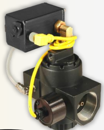
QB2 on PSR (volume booster) with DSY pressure transducer providing 2nd loop feedback
