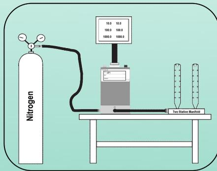
In this application a Proportion -Air GP high pressure device is being used to control the amount of pressure being applied to shape a catheter in a mold. The GP controls pressure up to 1000psi with 0.25% accuracy.
