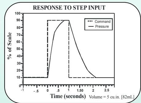
Times for GP to fill/exhaust a closed chamber. Step command signal is superimposed over pressure trace. Time is determined by difference between command signal and pressure achieved.
